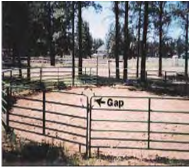
Typical 60-foot diameter portable panel round pen. Gaps can trap hooves and tails of animals
