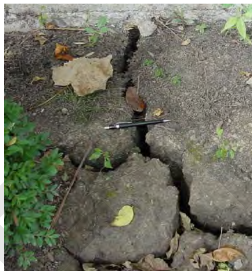
Expansive Soil Source: USGS Photo Gallery
